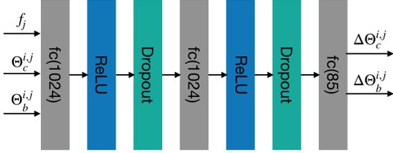
Figure 2: Detailed network structure of the regression block at the  $i^{th}$  stage and the  $j^{th}$  view.  $f_j$  denotes the image feature of the  $j^{th}$  view,  $\Theta_c^{i,j}$  denotes the camera parameters, and  $\Theta_b^{i,j}$  denotes the human body parameters.
